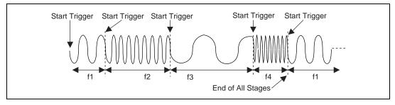
Figure 2-7. Stepped Trigger Mode
